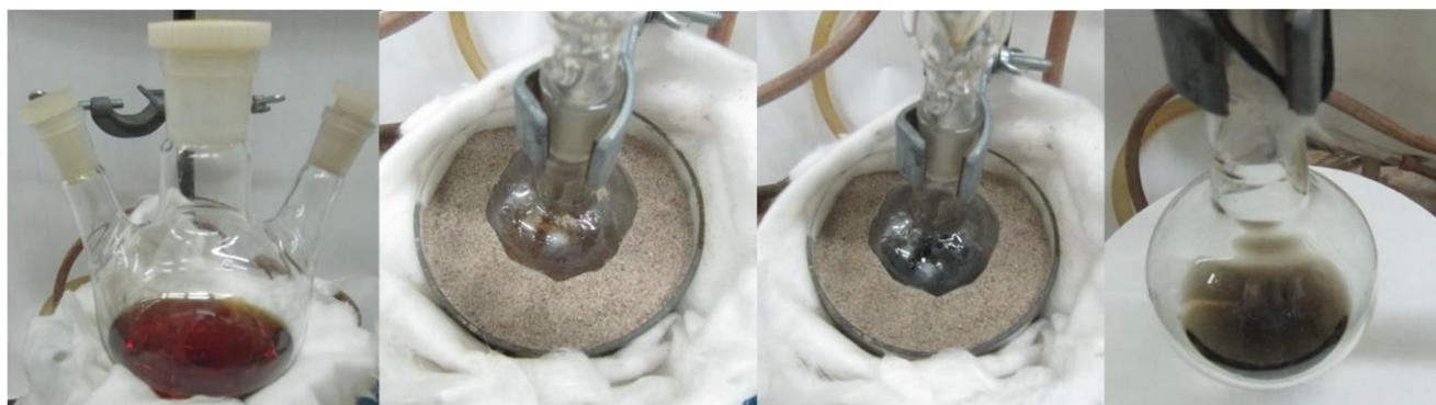
Figure 1. Change of color during reduction of the sample Ru-EG-5 under reflux conditions.
